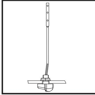
Enter the nut on the handle and tighten.
